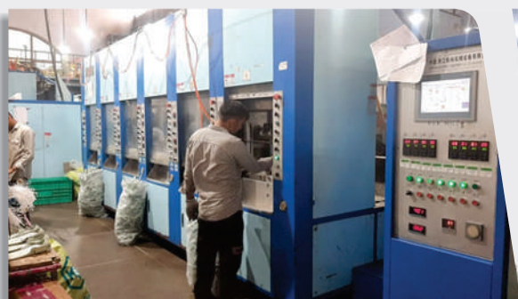
Our new EVA machines use Servo Controlled Hydraulic systems which reduce power consumption & wear & tear.
